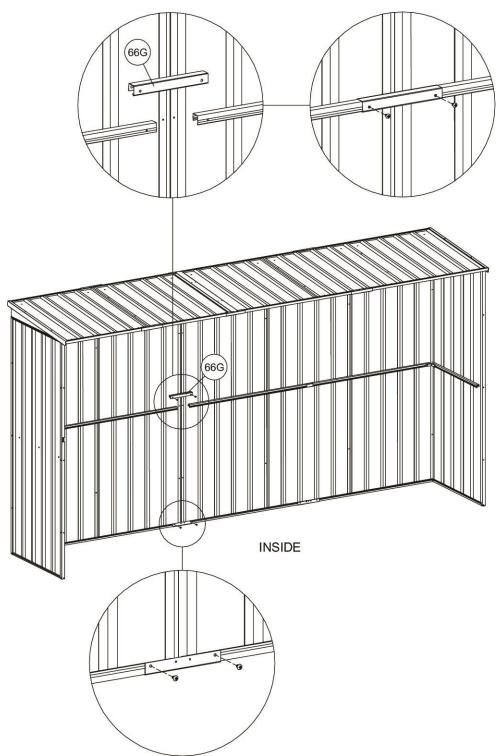
You are now ready to bolt down your shed. Refer back to the roof module instructions for how to bolt down your shed. Bolt down brackets can be flexibly placed to suit your position. You should try and position a bolt down bracket either side of the joiner, either side of a door opening and at equal distances on other walls.
