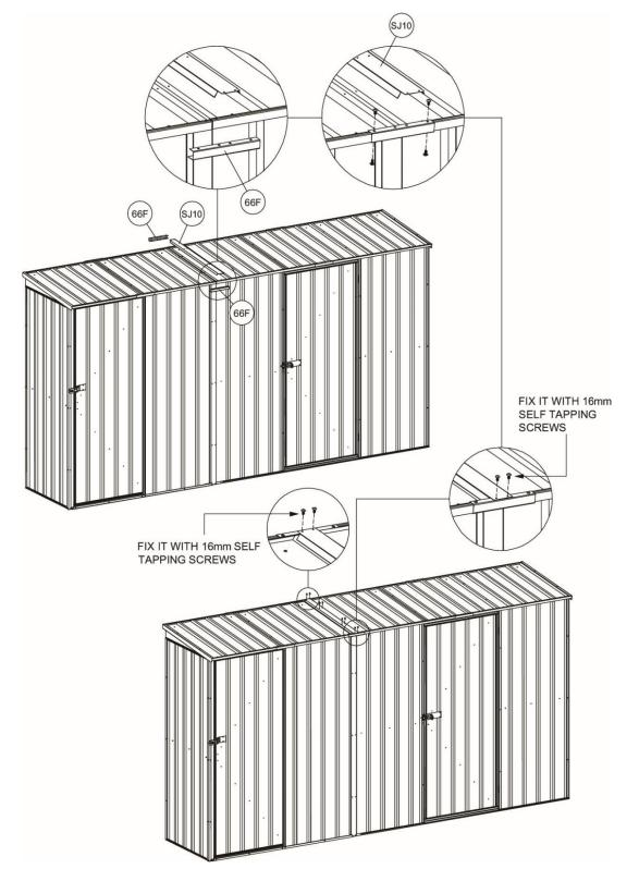
Now fit SG39 Gable infill piece as per the diagram. Fix with 16mm self-tapping screws. Now move inside the shed. Attach the Brace SB01 as per the diagram. When fixing to the joiner section use a 3mm drill to make a pilot hole from below, then secure with a 16mm self-tapping screw from the top.
