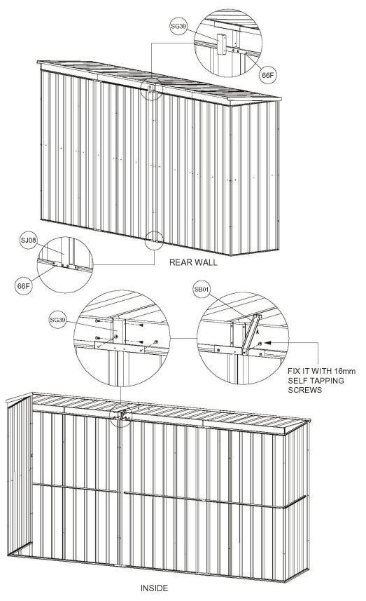
Fit 66G mid wall frame connector to back and front of shed as per the diagram Fix with 10mm selftapping screws
