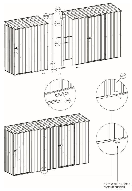
Place the 66F joiners on the roof channels as per the diagram. Place the SJ10 roof Jamb into
